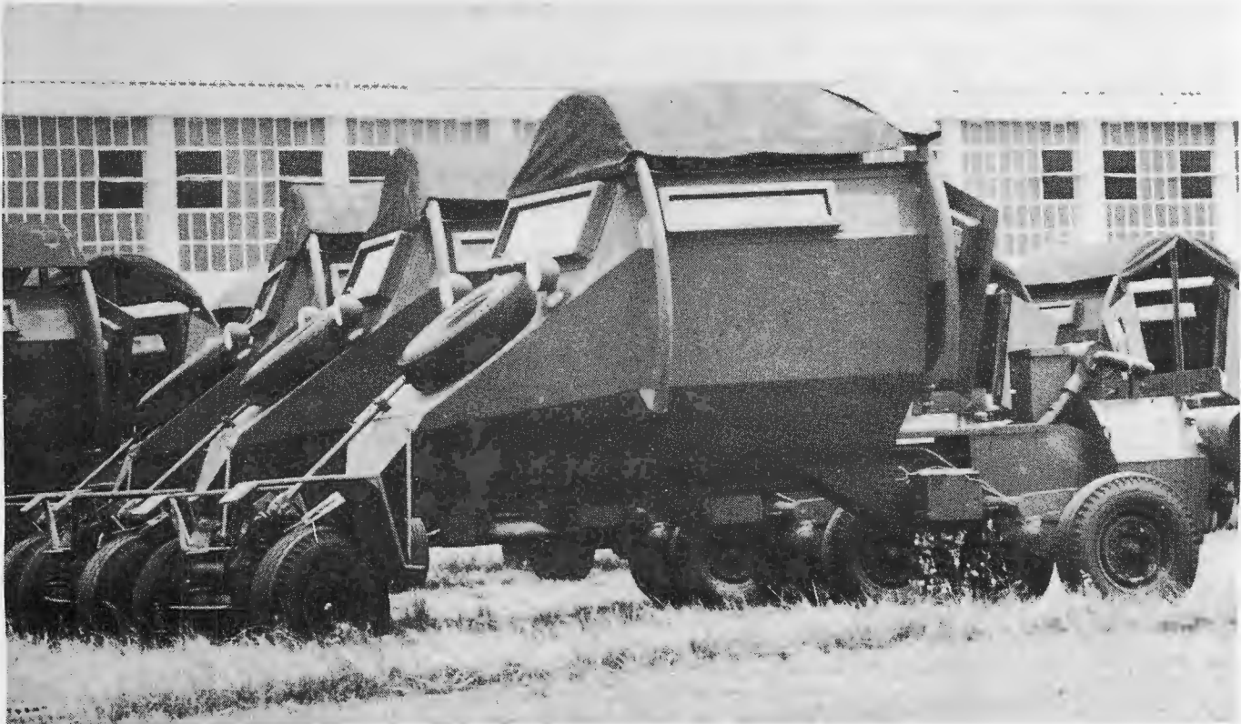
World-wide embargo on Rhodesia has resulted in unique improvisation on part of Rhodesians. Above are Rhodesian-made "Leopards," a vehicle designed for operation in the bush. Personnel compartment provides protection from blast if one of wheels hits mine.
